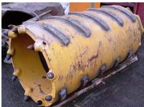
Round Shank Core Barrel (for medium hard to hard rocks)
