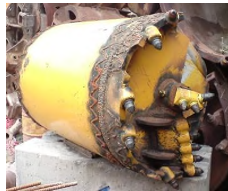
Rock Boring Bucket (for medium hard to hard rocks)
