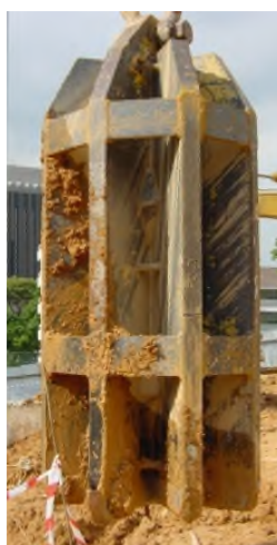
Chisel (for hard to very hard rocks)
